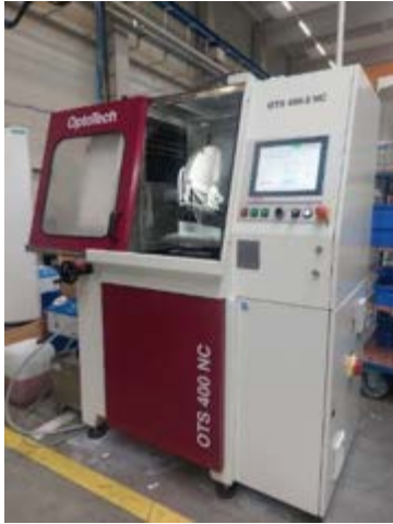
Cutting Machine Semi-automatic sawing process with NC
