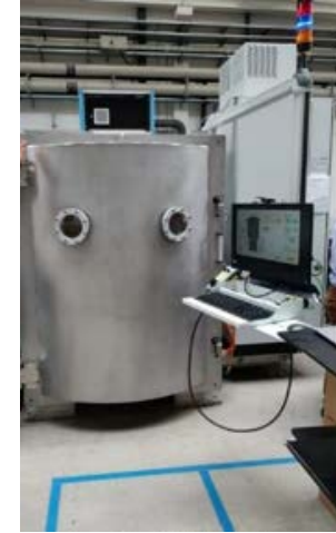
Ion Beam Figuring Surface errors < \lambda/200 – Dry polishing
