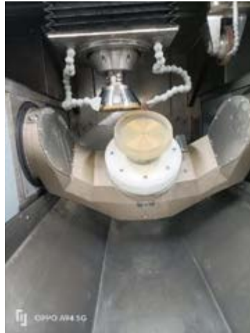
Grinding Machine Aspherical, spherical, prisms, cylinders, 3D optics
