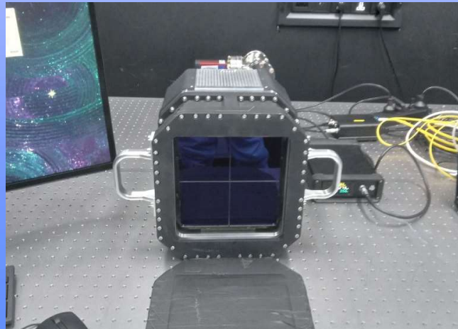
Gpixel GENS 2 x 2 mosaic of 9k x 9k x 10μm CMOS chips
